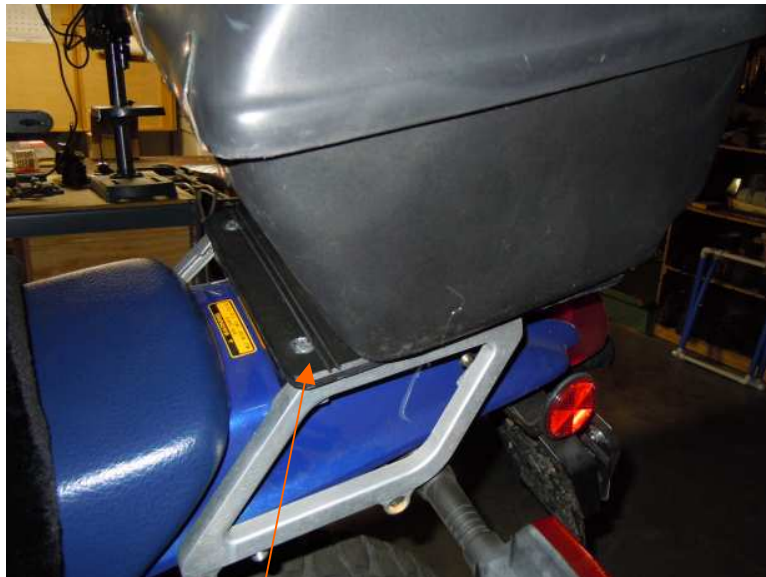
Offset to allow seat removal
