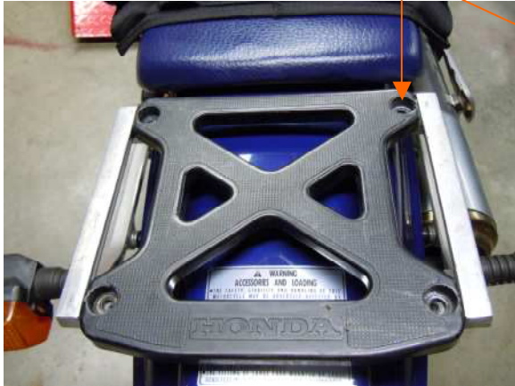
Rear Luggage rack on NX250 Adaptor "board" Mtg. Holes.
