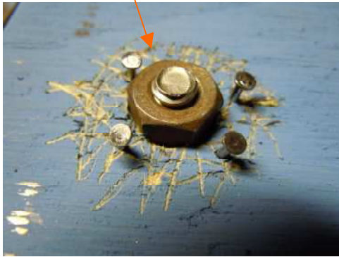
Detail of nuts epoxied to board Roughened surfaces on board and nut
